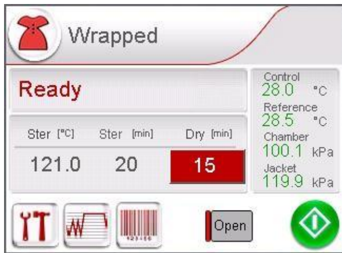
Operators Control Panel (Touch Screen)
